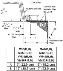
Figure 6 - Side Clearances - Top View (Cross Section)
